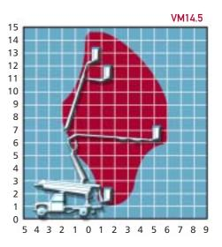
The VM10.5 and VM14.5 models are vehicle mounted work platforms suitable for mounting on chassis with minimum gross vehicle weight of 3050kg (VM10.5) and 3500kg (VM14.5).
